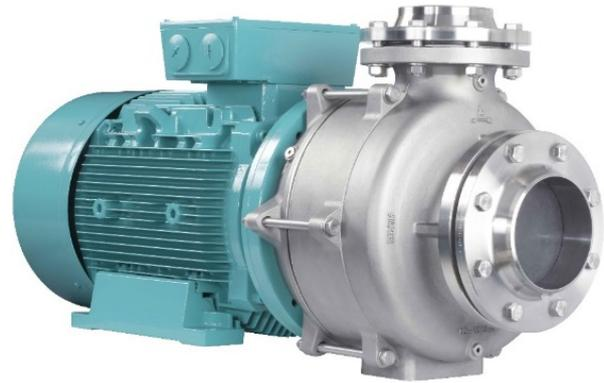
A torque-flow pump in compact bloc-design for the transport of liquids contaminated with solids or suspensions. Typical liquids are: waste water, cooling agents contaminated with metal chips, abrasive oils and lyes, lime milk and products that have to be transported with care.
